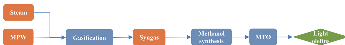
Figure 5. Simple block diagram of PMTO.
