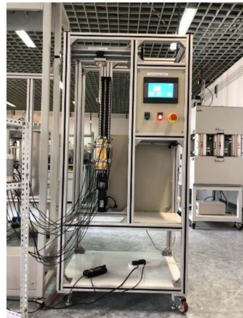
Figure 3. The automatic control system used for controlling movement of sensors and measured models in the ECT system.
