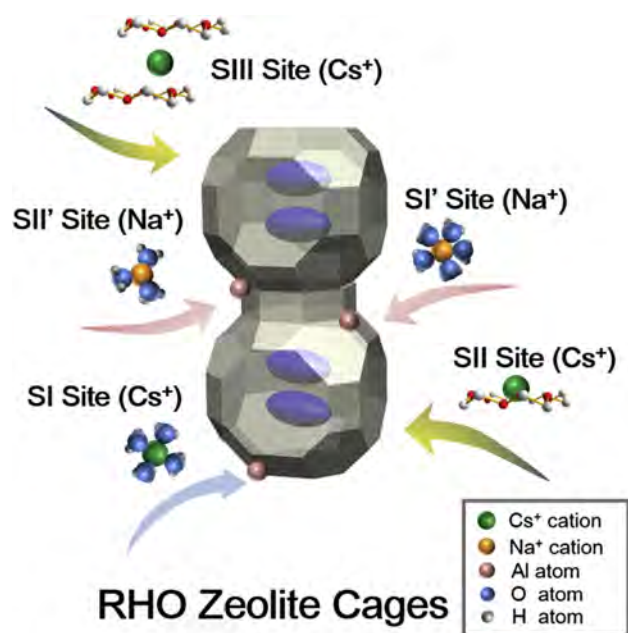
Fig. 4. Schematic description for the assignments of resonance peaks in the ^{133}\text{Cs} and ^{23}\text{Na} MAS NMR spectra of the as-made RHO zeolites. (SI: fully hydrated \text{Cs}^+ cation, SII: \text{Cs}^+ -crown ether monomer complex, SIII: \text{Cs}^+ -crown ether dimer complex; SI': fully hydrated \text{Na}^+ cation, SII': partially hydrated \text{Na}^+ cation.)
