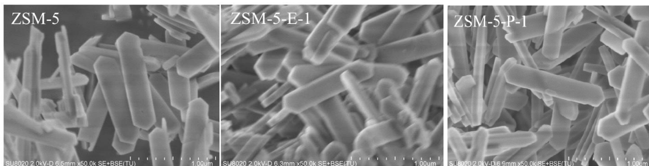
Fig. S2. SEM images of ZSM-5 zeolites before and after post-synthetic treatment.
