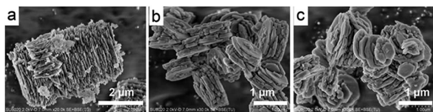
Fig. 7 SEM images of CrAPO-5-NS (a), CoAPO-5-NS (b), and MnAPO-5-NS (c).
