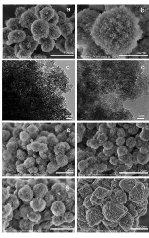
Fig. 3 SEM images of samples 3 (a and b), 13 (e), 14 (f), 15 (g), commercial beta (h) and TEM images of sample 3 (c and d).
