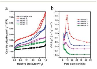
Fig. 2 N<sub>2</sub> adsorption-desorption isotherms (a) and pore size distribution curves from the adsorption branches (b) of the samples (the isotherms of sample 3 were vertically offset by 100 cm<sup>3</sup> g<sup>-1</sup>).
