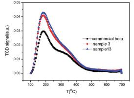
Fig. 8  $NH_3$ -TPD curves of sample 3, sample 13 and commercial beta.
