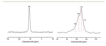
Fig. 4  $^{27}$ Al and  $^{29}$ Si MAS NMR spectra of the as-synthesized beta (sample 3).
