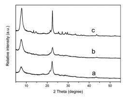
Fig. 1 XRD patterns of the as-synthesized sample 3 (a), calcined sample 3 (b) and commercial beta (c).
