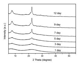
Fig. 6 XRD patterns of the as-synthesized samples with different crystallization time (the initial gel has the same molar composition as that of sample 3).
