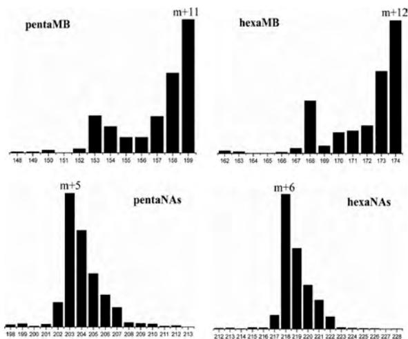
Fig. 6 Isotopic distributions of the retained organic material after co-feeding <sup>13</sup>C methanol and 1 wt% <sup>12</sup>C naphthalene at 250 °C for 20 min.
