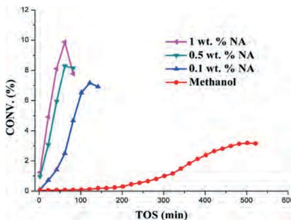
Fig. 2 Methanol conversion profiles as a function of TOS for methanol co-feeding with different profiles of naphthalene at 250 °C on the HZ-19 catalyst.
