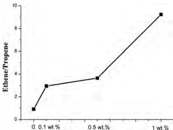
Fig. 4 Ethene/propene ratios at different feeding conditions when methanol conv. = 1% at 250 °C for the HZ-19 catalyst.
