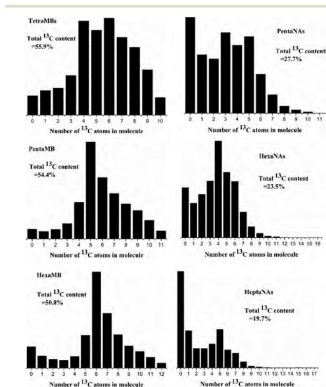
Fig. 8 Isotopic distributions of the retained organic materials after the <sup>12</sup>C/<sup>13</sup>C switch experiment at 250 °C: co-feeding <sup>12</sup>C-methanol and 1 wt% naphthalene for 40 min during the MTH reaction, followed by 2 min of <sup>13</sup>C-methanol feeding. The total <sup>13</sup>C content of each molecule was marked in each picture.
