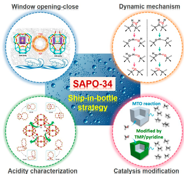
Figure 1. Ship-in-a-bottle strategy for acidity characterization and SAPO-34 catalyst modification for MTO reaction. Adapted with permission from ref 48. Copyright 2020 Wiley-VCH GmbH.
